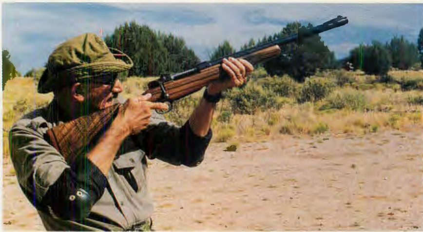
SOF's Technical Editor, Peter Kokalis, aka "Rice Paddy Daddy," fires a center-of-mass hit on a 75-yard Pepper Popper with "Baby IV," more-or-less a duplicate of Jeff Cooper's "Baby" — built from a highly modified Czech Brno ZKK 602 and chambered for the massive .460 G&A cartridge. Photo: Gabe Suarez
